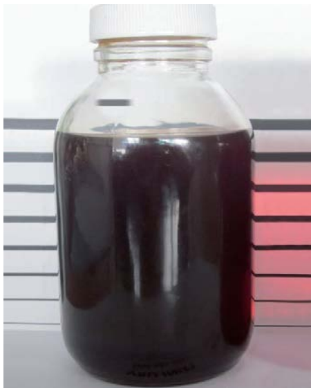
Gas Turbine Oil with Varnish
