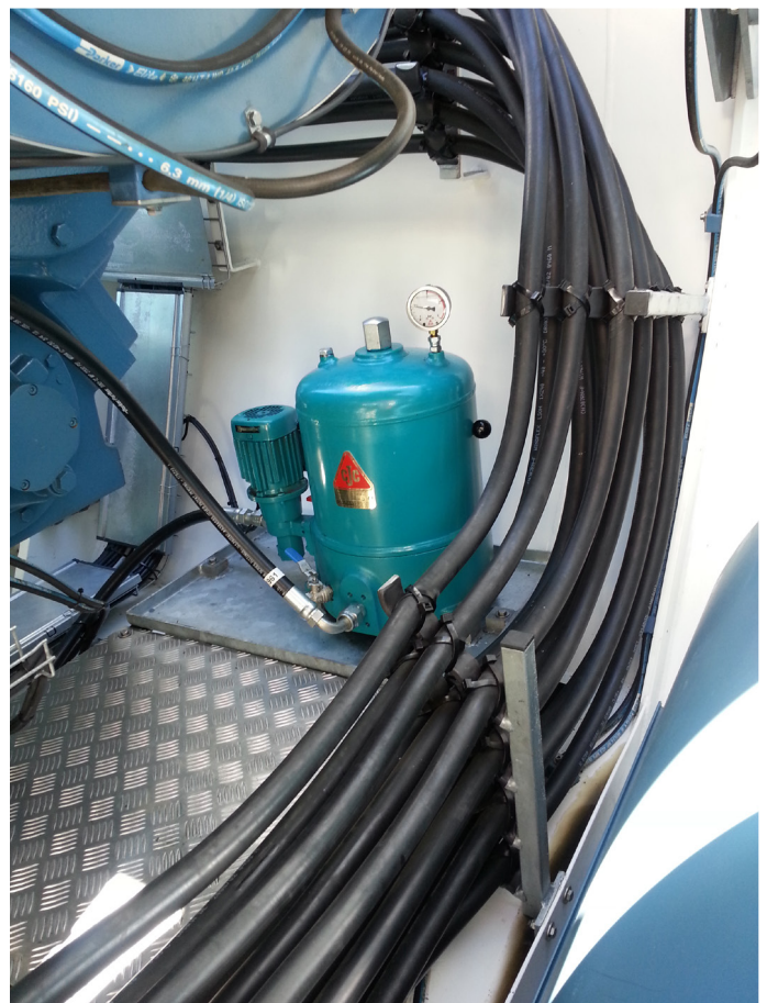
Figure 13 Offline and inline filters are common in the wind industry and provide the optimum level of contamination control.
