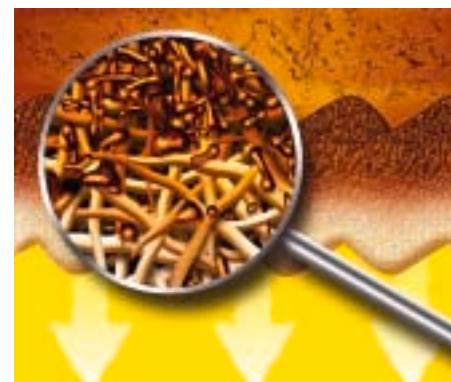
Adsorption of oxidation by-products in the CJC™ Fine Filter: Resin in the oil attracts to the polar fibres in the filter mass and are retained
