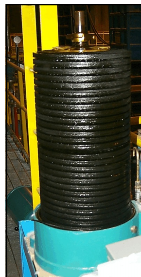
III. 2: The CJC Filter with housing dismantled. After 6 months of operation. The dark, shiny colour of the filter inserts indicates oxidation products.
