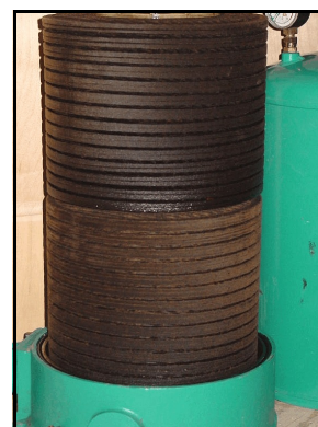
III. 3: The CJC Filter Insert after 12 months' test (6 months after insert replacement). When compared with ill. 2 it is clear that the oil was more clean during the last 6 months of the test, thus depositing less of the brown oxidation products.
