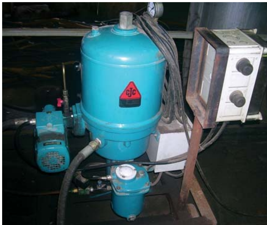
Figure 2. This water separator unit utilizes the coalescing principle coupled with a fine-depth cellulose filter with Beta 3 > 75 to remove particles and emulsified water.
