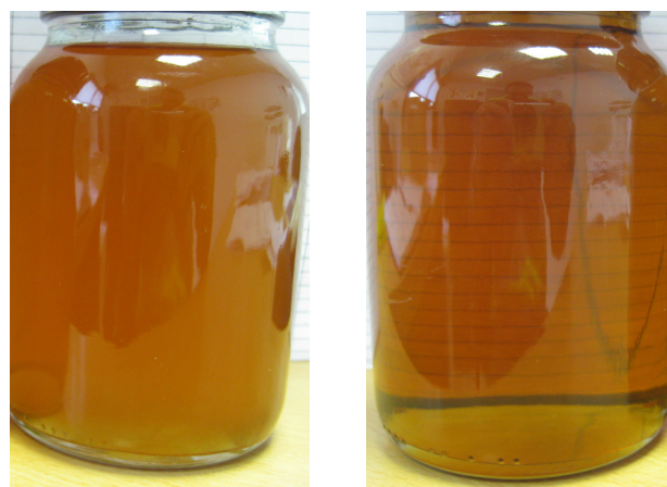
Appearance of the oil after sampling at the CJC® VRU Filter - Inlet & Outlet.
