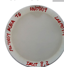
Membrane Patch AFTER 6 months operation
