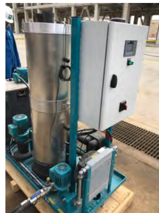
The varnish removal unit utilized by Saudi Aramco. Courtesy: CJC
