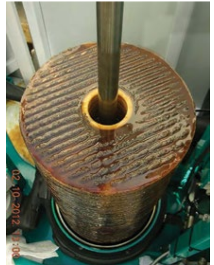
2. Filter disks are effective in removing varnish
