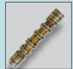
Varnish on valve spool
