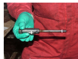
Wear on injector - risk of leakage
