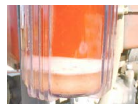
Bacteria growth - risk of blockage of filters
