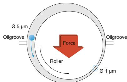
Figure 1: Lubricating a journal bearing
