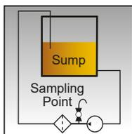
If no offline filter system is installed, a vacuum type sampling pump is a valid option. In such case the sample should be drawn 10 cm (4 inches) off the lowest part of the tank (see page 18).
