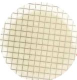
Contaminated Millipore membrane. Sample taken before offline filtration.
