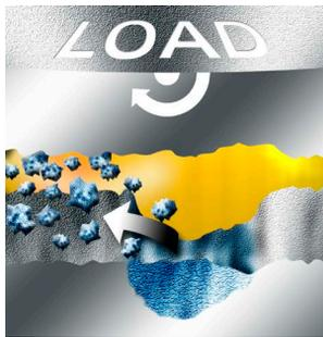
Figure 3: Fatigue Wear
