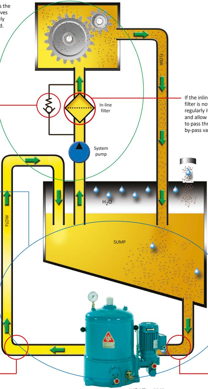
If the inline filter is not changed regularly it will clog and allow particles to pass through the by-pass valve.
