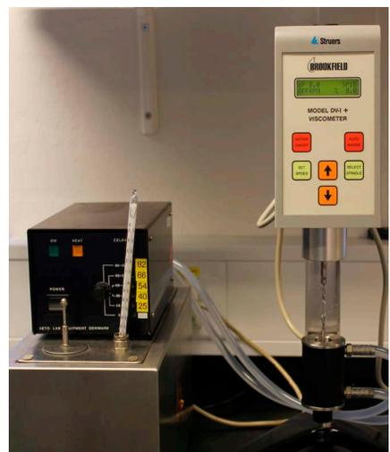
Figure 14: Equipment to test dynamic viscosity (cP)
