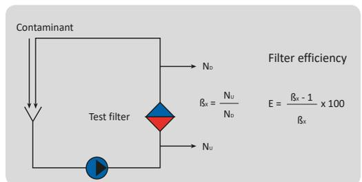
Figure 26: Multipass test
