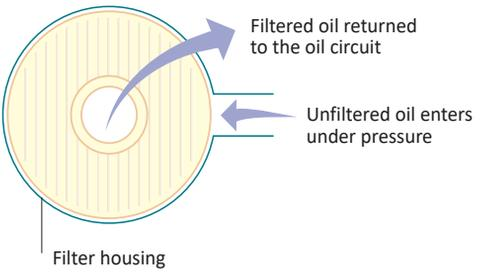
The CJC® Offline Oil Filter has a large dirt holding capacity of approximately 4 L solids, up to 2 L of water and 4 L oil degradation products (varnish). The CJC® Offline Oil Filters typically only need replacing every 12 months.
