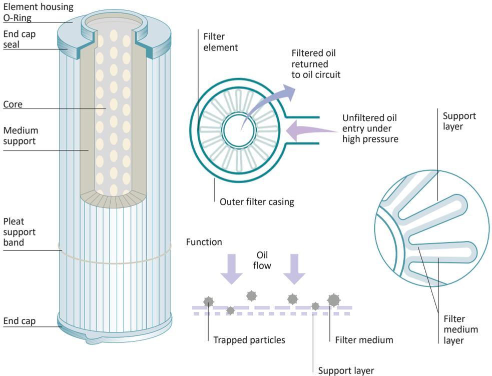
Pressure filters have a limited dirt holding capacity, usually between 1 and 100 grams, which results in filter element replacement at short intervals in order to ensure efficient filtration.
