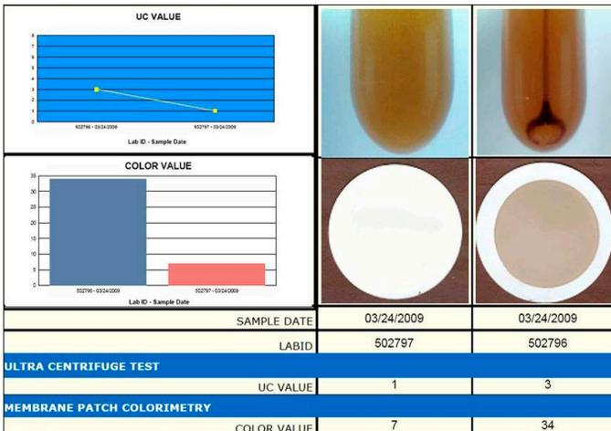
Figure 24: UC Analysis and MPC Test Result
