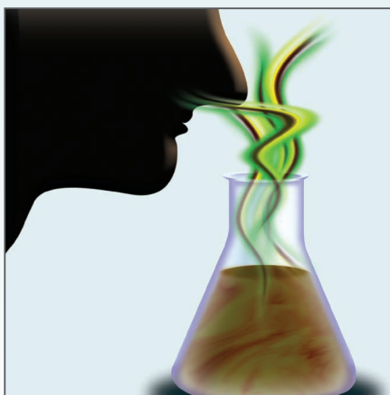
Sour and putrid odour indicates oil degradation
