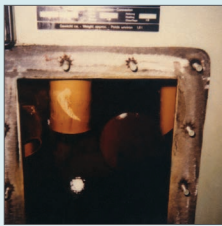
Oil reservoir on plastic moulding machine
