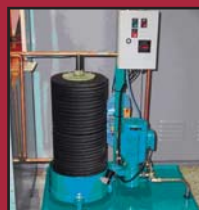
Figure 5. Governor Filter Varnish Removal
