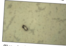
Oil sample taken BEFORE installation of CJC™ Oil Filter ISO 20/18/15
