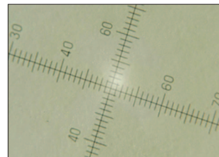
Oil sample no. 3, 12th Okt. 2007: AFTER 4 weeks of fine filtration result: ISO Code 13/12/9
