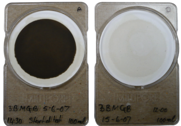
Before and after patch tests. After a trial period of 10 days - ISO Code - / 15 / 13
