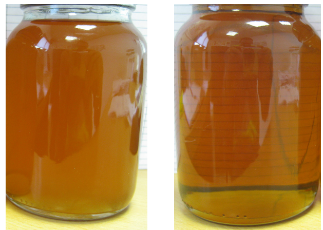
Appearance of the oil after sampling at the CJC® VRU Filter - Inlet & Outlet.
