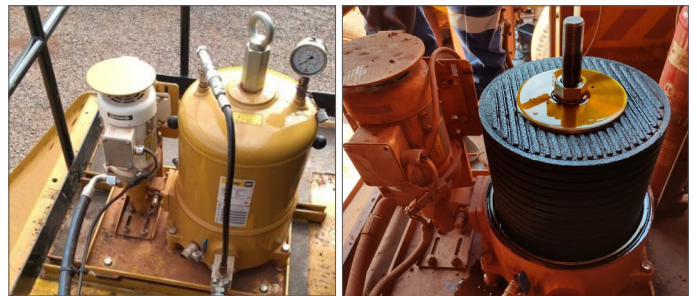
One of the CJC® Oil Filters installed at the 6 haul trucks.
