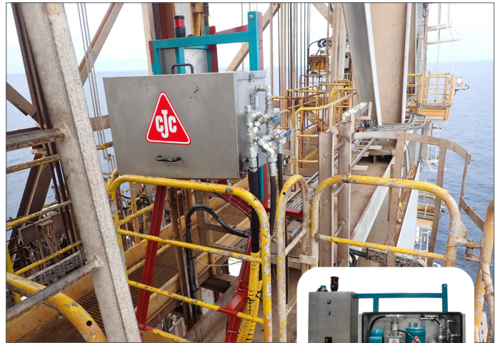
The CJC® HDU 15/25 installed at the drilling derrick of the drill tower.
