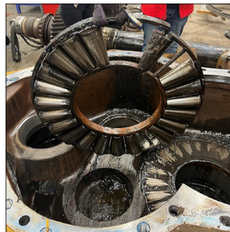
Defect Top Drive gearbox due to contaminated oil
