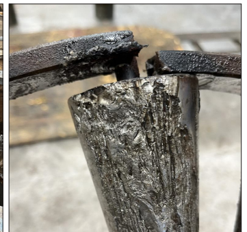
Defect Top Drive gearbox due to contaminated oil
