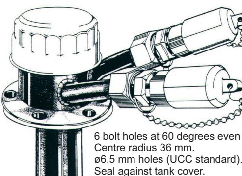
Plastic tap, identifying suction connection (pipe from tank bottom).
