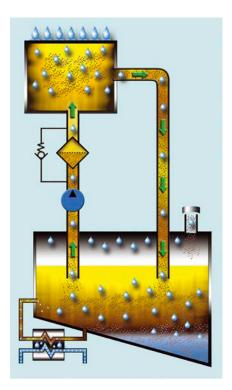
Typical system with no off-line filtration
