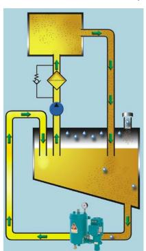
System with continuous off-line filtration
