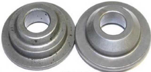
Figure 6. Part on the left is from a system before a fine filtration system has added. You can see the deposits of carbon. The picture on the right was from the same quenching system after fine filtration was installed.
