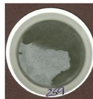
Before Offline Filter Installed: ISO 19/16/13 = DIRTBOX
