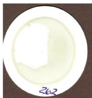
After Offline Filter Installed: ISO 15/12/10 = GEARBOX
